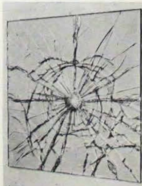
Rolling sheets into safety glass. Below — it may crack but it won't fall apart.
